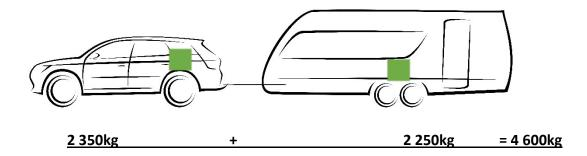
If the vehicle is loaded to maximum, then: 4600 kg - 2740 = 1860 kg maximum allowable trailer load.
