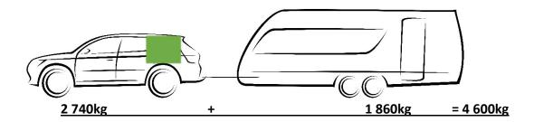
In this instance, the vehicle is loaded to maximum and the trailer is loaded to maximum. The total weight has exceeded the allowable limit.
