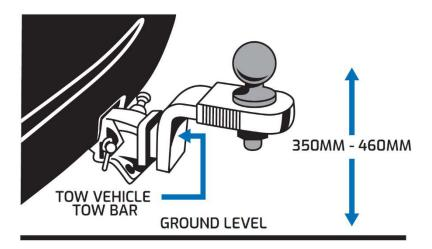
The most commonly used 50mm diameter tow balls are not rated beyond 3,500kgs. Towing 3,500kgs to 4,500kgs requires the use of a 75mm tow ball or other coupling rated to the ATM of the trailer.
