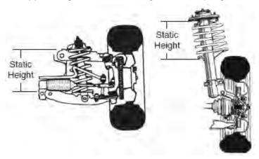
still in the vehicle while the body of the vehicle jacked up, to full extension of shock absorber.
